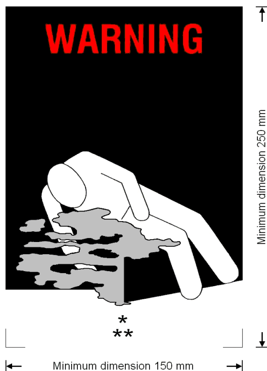
Coolant/conditioning warning mark for cargo transport units
