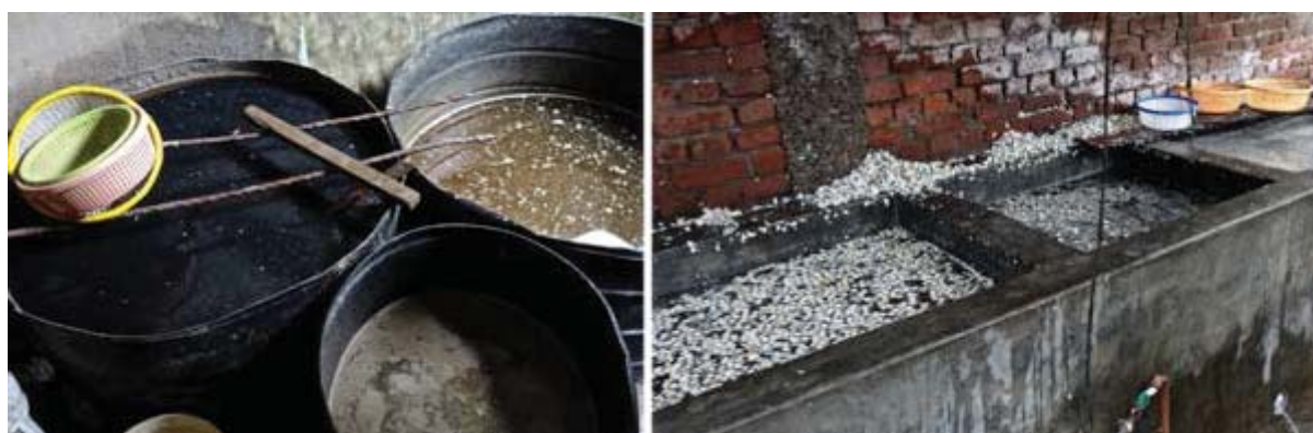
Figure 14: Multi-step density separation using the sink/float method
