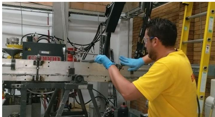
Figure 5. Measurement of foam expansion at Brett mould
